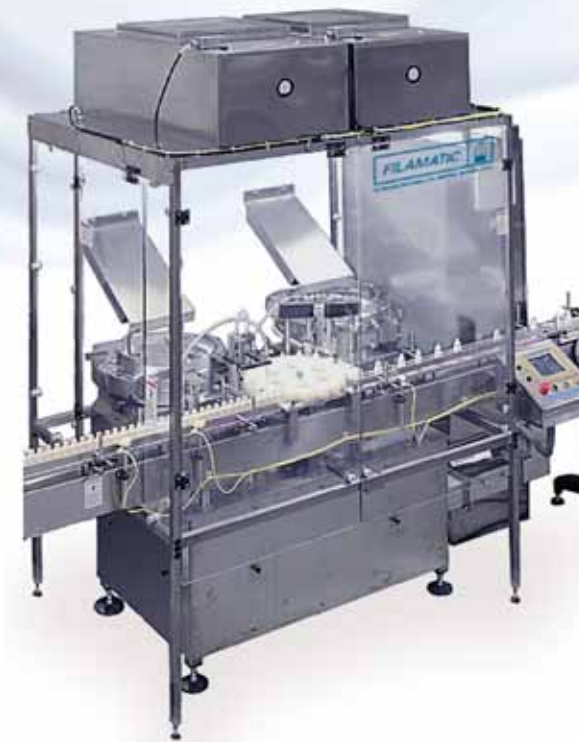
MNB 2000 A complete fill/finish packaging system
